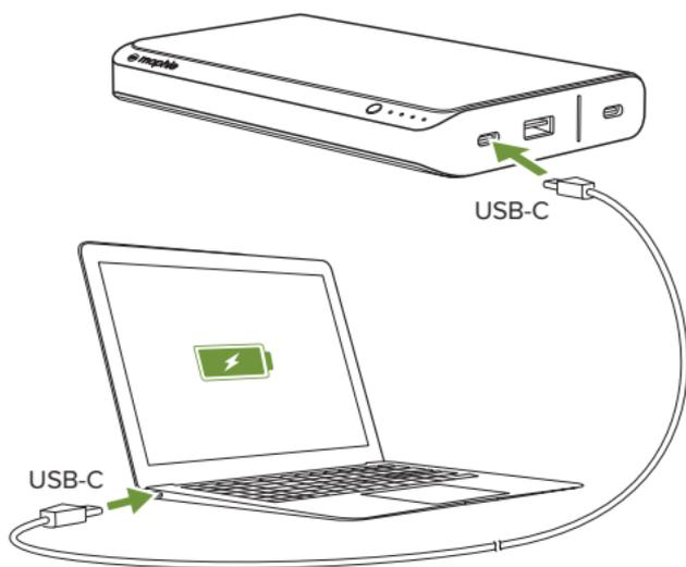
**IMPORTANT:** Do not connect a USB-C equipped laptop to the **powerstation pro XL** battery's USB-A port.
